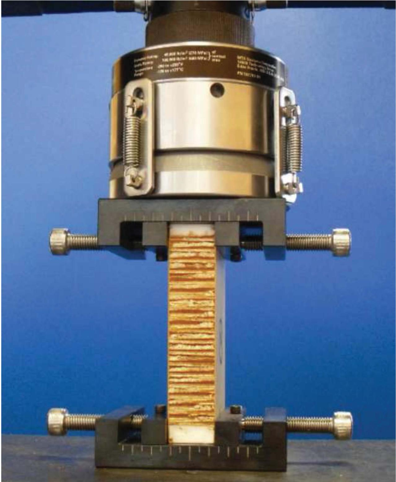
Figure 5. Configuration for static edgewise compression experimental tests.
