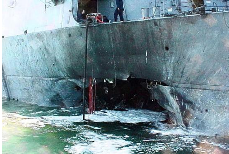
Figure 2.8 Hull damage in USS Cole. Photographs from US Navy archives [7].
