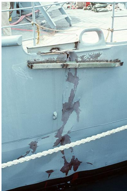
Figure 2.9 Cracked hull of USS Princeton. Photographs from US Navy archives [8].
