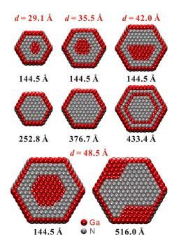
FIG. 3. (Color online) Inversion domain boundary distributions in GaN nanorods of different lateral dimensions (d) and lengths (below each pattern).
