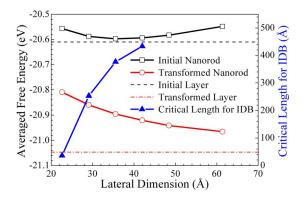
FIG. 4. (Color online) Average free energies per atom for the initial and transformed configurations of GaN layers and nanorods of the same length (144.5 Å) at different lateral dimensions, also shown is the critical length below which the IDB is observed in GaN nanorods.
