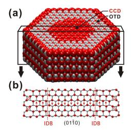
FIG. 2. (Color online) (a) Section of GaN nanorod with two wurtzitestructured domains [the core columnar domain (CCD) and the outer tubular domain (OTD)] separated by an inversion domain boundary (IDB); (b) atomistic arrangement on  $(01\overline{10})$  cross-section showing the structure of the IDB.
